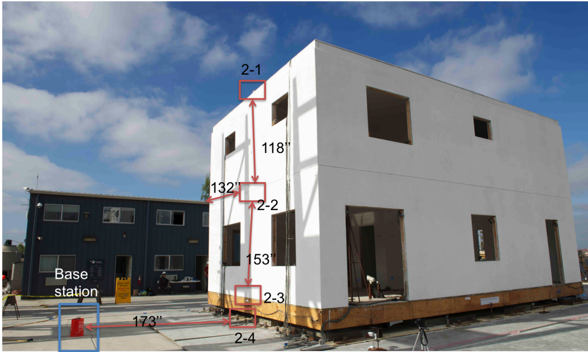
Figure 6: Sensor location on the East side wall with the distances.
