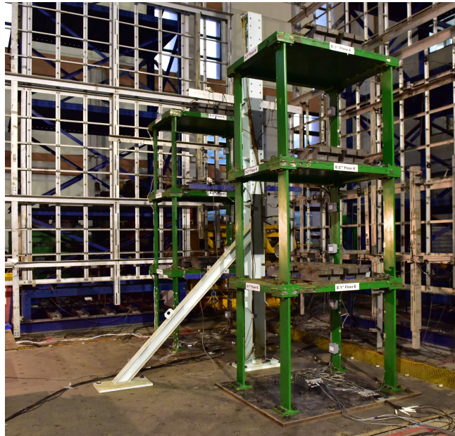
Figure 3. Photo of two structures (in green) on the shake table. The front structure is Specimen 1 and the back structure is Specimen 2.
