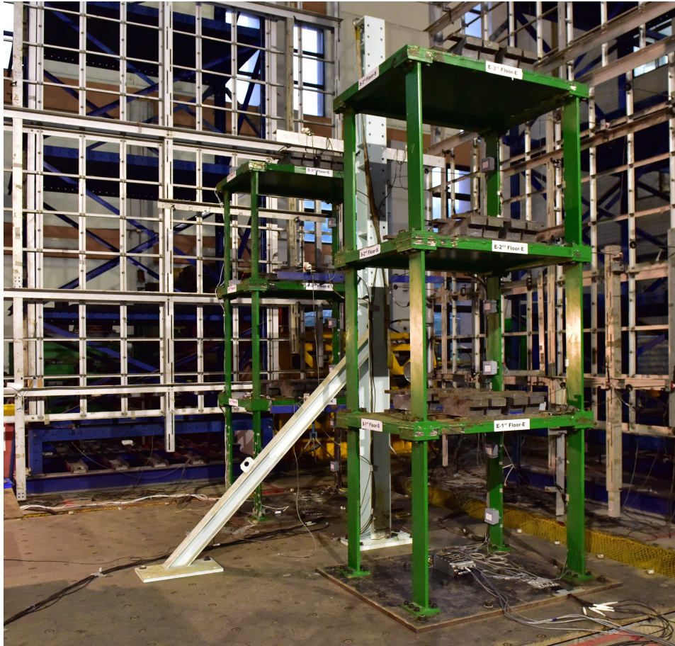
Figure 2: Photo of two structures (in green) on the shake table. The front one is Specimen 1 and the back one is Specimen 2.
