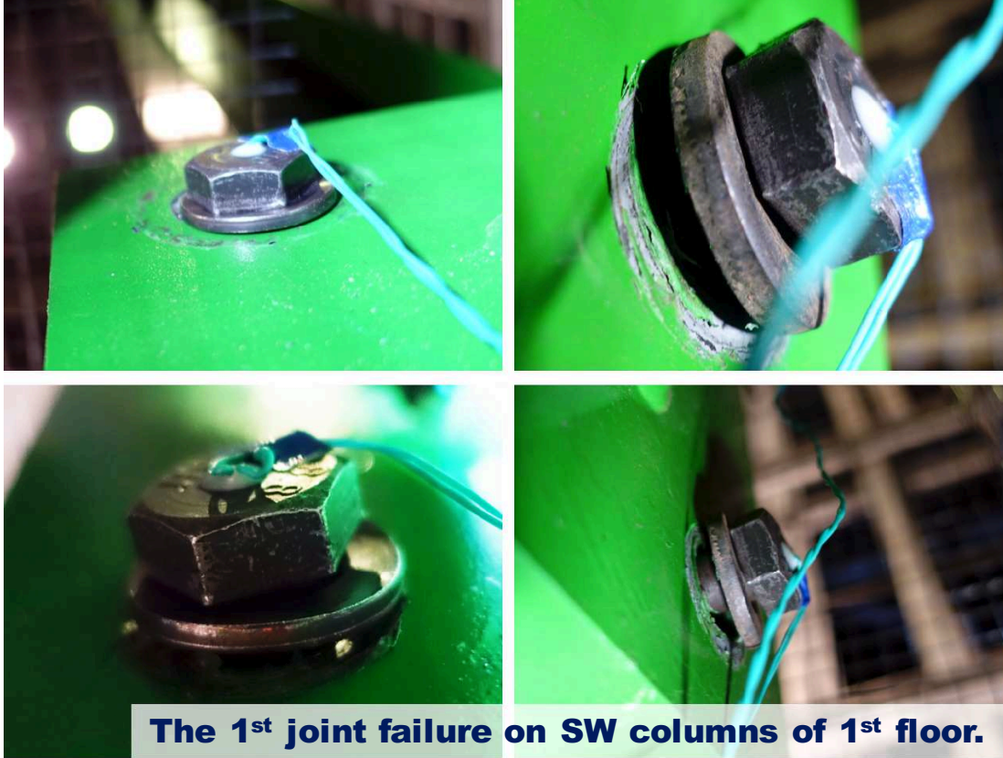
Fig. 9. Experiment 2: washers and bolts after 0.7g strong motion excitation.
